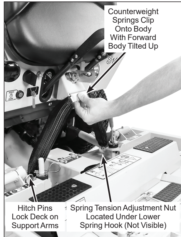
Deck Counterweight Spring Installation
