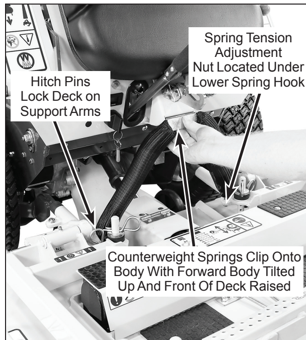
Deck Counterweight Spring Installation
