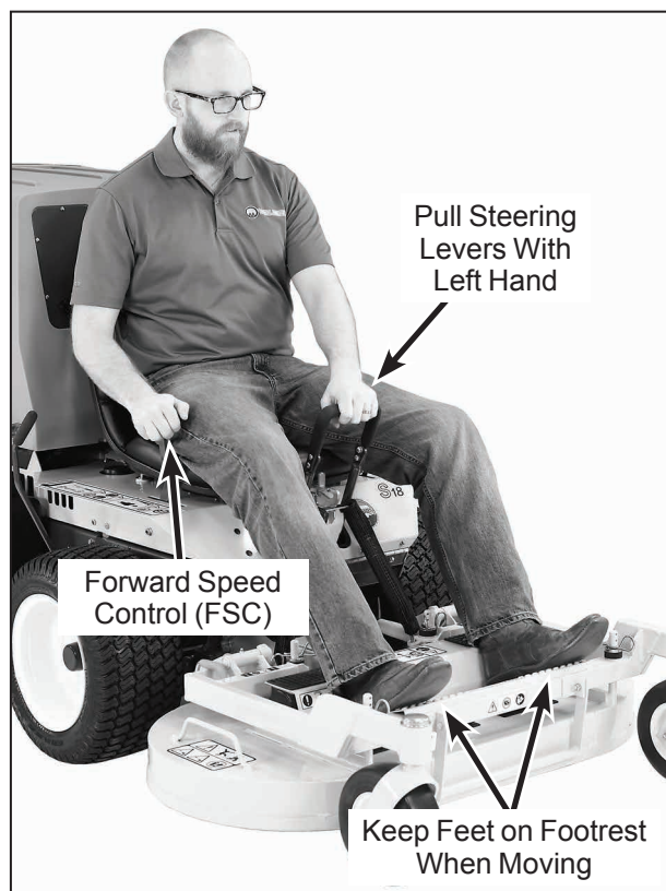
Correct Operator Hand Position on the Controls
