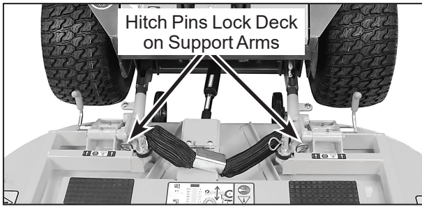
Use Hitch Pins to Lock Deck on Support Arms
