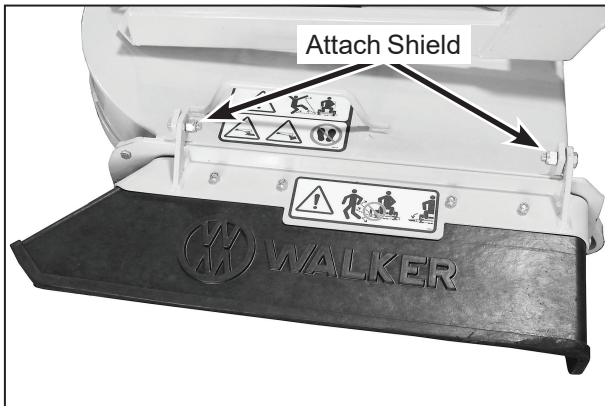
Deck Discharge Shield Installation
