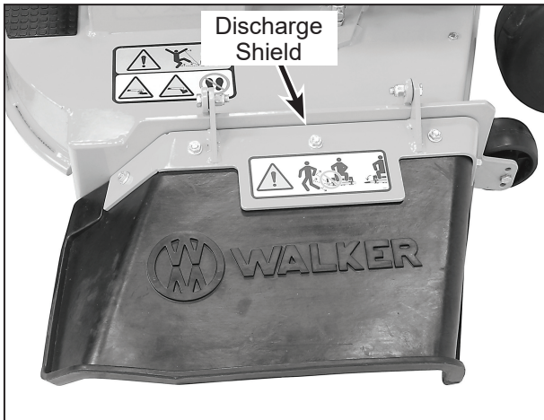
Side Discharge Deflector Shield in Lowest Position
