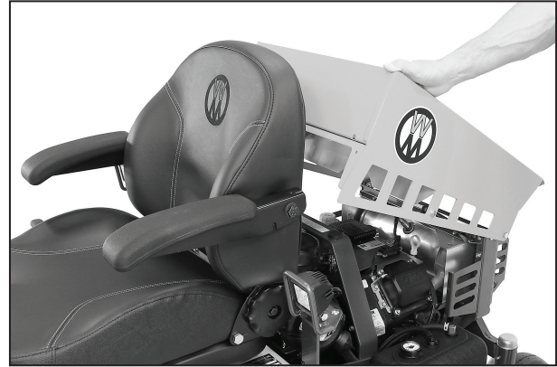
Lifting Utility Bed
