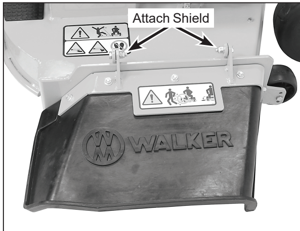
Deck Discharge Shield Installation
