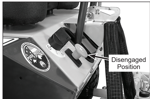
Blade Clutch Disengaged
