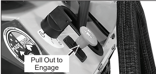
Blade Clutch Engaged
