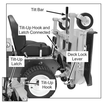
**Deck Secured in TILT-UP Position**
