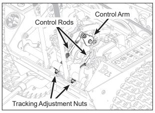
**Transmission Control Rod and Arm Location** (Components Hidden for Clarity)
