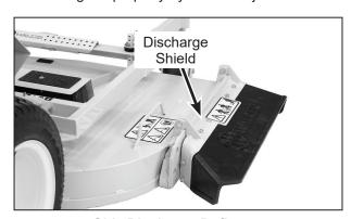
**Side Discharge Deflector Shield in Lowest Position**
