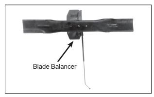
Blade Balanced on Magnetic Wall-Mounted Balancer
