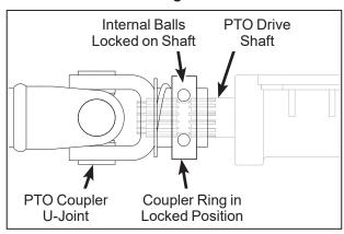
**Quick Disconnect Ring "Locked" Position**
