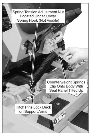
**Deck Counterweight Spring Installation**
