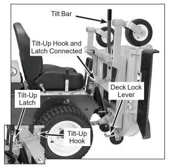
**Deck Secured in TILT-UP Position**
