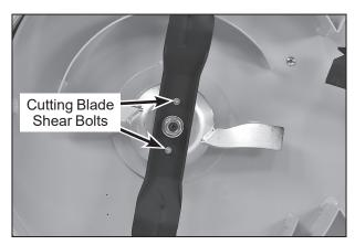
**Cutting Blade Shear Bolts**
