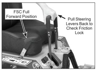
FSC Friction Adjustment Test (Checking Friction Lock)
