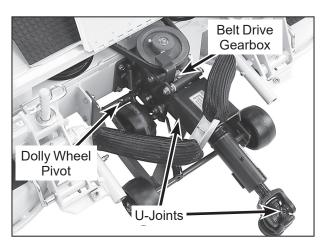
Gearbox, Dolly Wheel, and U-Joint Lubrication
