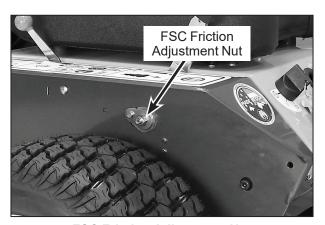
**FSC Friction Adjustment Nut**
