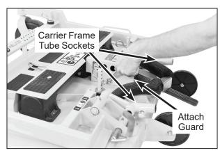
**PTO Shaft Guard Installation**
