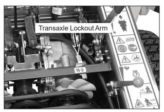
Transaxle Lockout Arm - Freewheel Position
