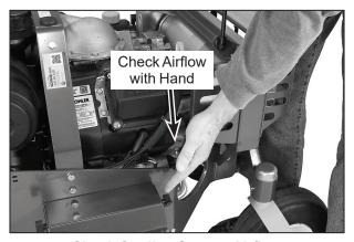
**Check Cooling System Airflow**
