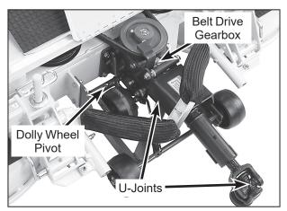
Gearbox, Dolly Wheel, and U-Joint Lubrication
