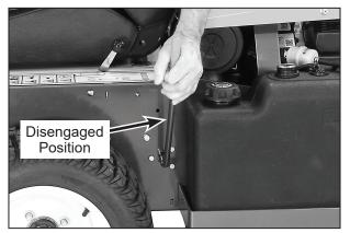
Parking Brake Disengaged
