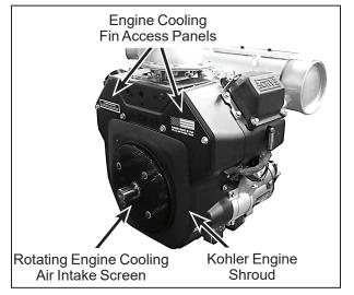
Engine Cooling Air Intake Screen and Cooling Fin Access Panels
