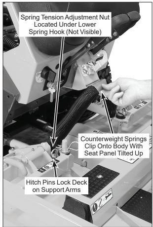
Deck Counterweight Spring Installation
