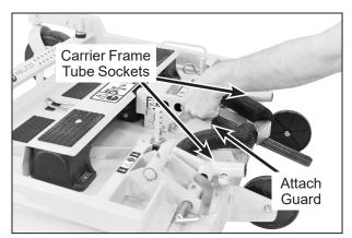
**PTO Shaft Guard Installation**
