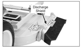
Side Discharge Deflector Shield in Lowest Position
