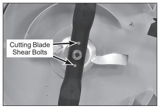
**Cutting Blade Shear Bolts**
