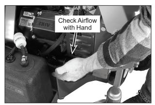
**Check Cooling System Airflow**
