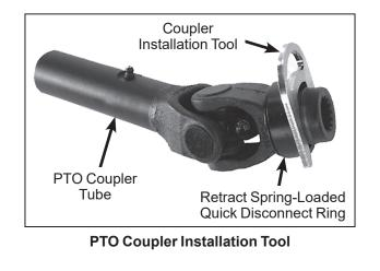
Reaching under the tractor, slide the PTO coupler tube onto the deck drive shaft (align arrow decals), then install the coupler quick disconnect onto the tractor PTO drive shaft.
