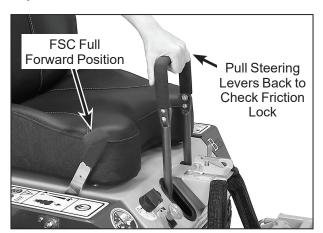
FSC Friction Adjustment Test (Checking Friction Lock)
