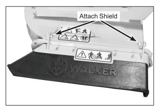
Deck Discharge Shield Installation
