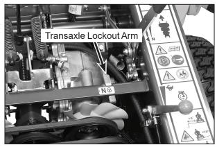
Transaxle Lockout Arm - Normal Operating Position
