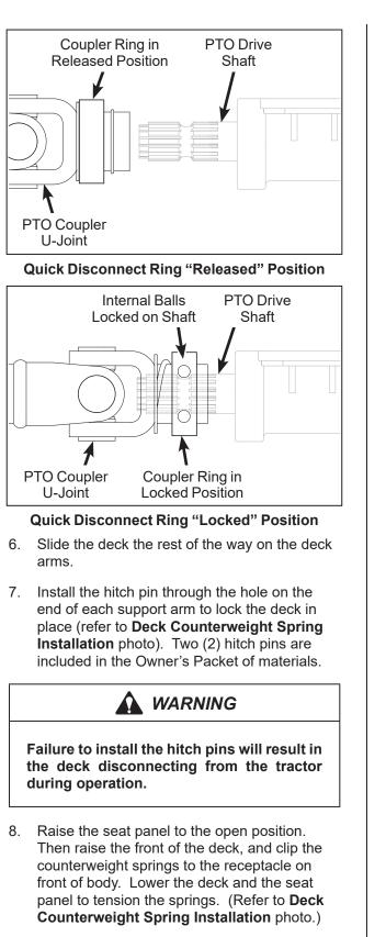
9. With the counterweight springs connected, the weight on the deck caster wheels should be 15 to 25 lb (6.8 to 11.3 kg); this adjustment is preset at the factory. If required, the spring tension can be adjusted by tightening or loosening the elastic stop nuts located underneath the lower spring hook, or contact your local dealer if additional help is required. Refer to **Deck Counterweight Spring Installation** photo.
