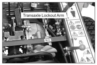
**Transaxle Lockout Arm - Freewheel Position**
