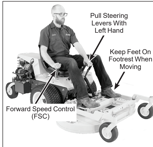
Correct Operator Hand Position on the Controls
