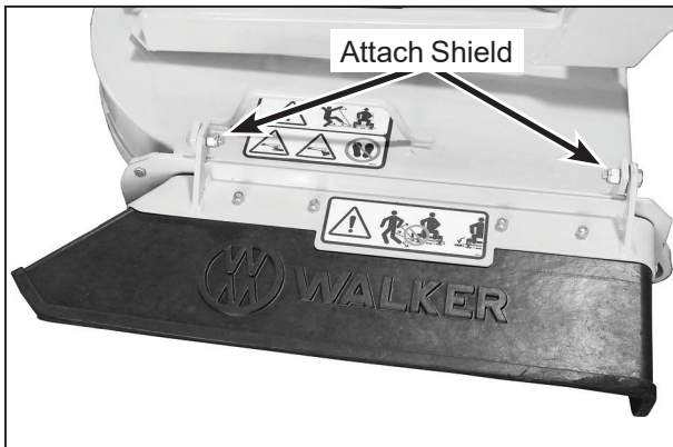
Deck Discharge Shield Installation
