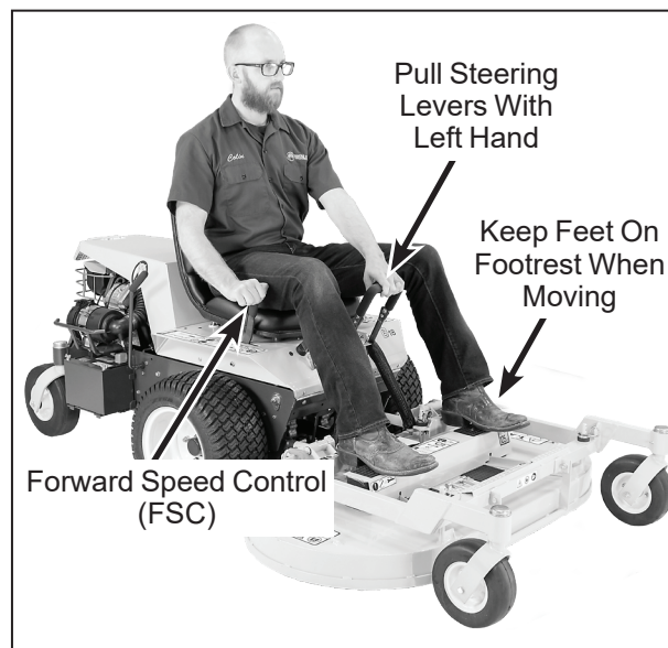
Correct Operator Hand Position on the Controls
