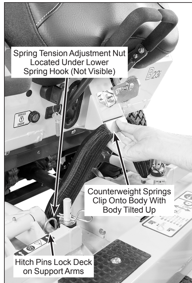
Deck Counterweight Spring Installation
