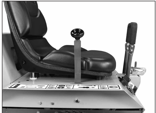
Correct FSC Lever NEUTRAL-PARK Position
