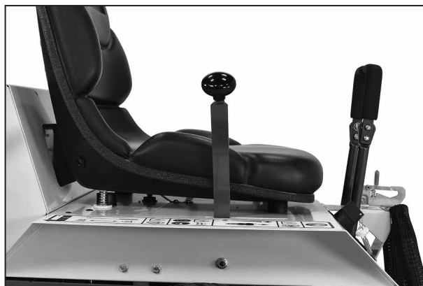
Correct FSC Lever NEUTRAL-PARK Position
