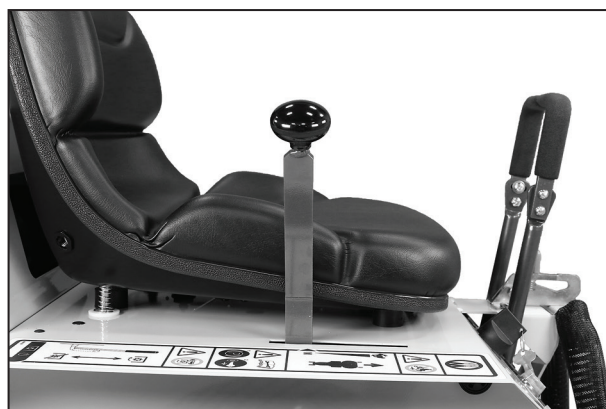
Correct FSC Lever NEUTRAL-PARK Position
