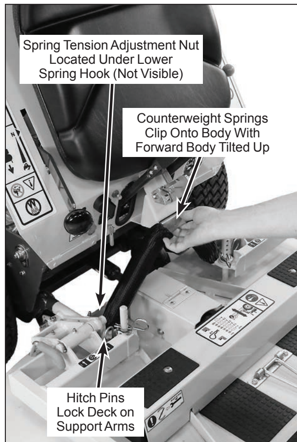
Deck Counterweight Spring Installation
