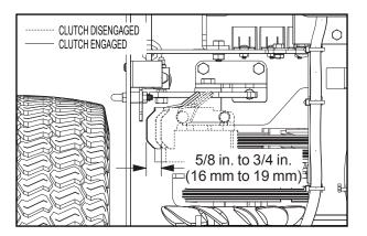
**Clutch Idler Pulley Travel Adjustment**
