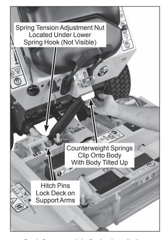
Deck Counterweight Spring Installation
