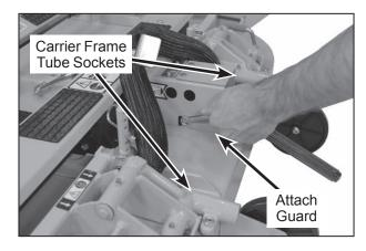
**PTO Shaft Guard Installation**
