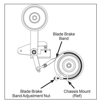
**Blade Brake Band Adjustment**
