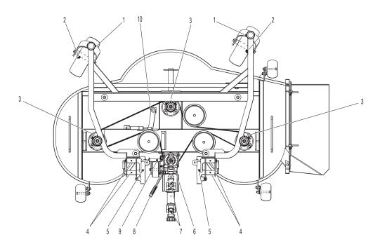
**Lubrication Points for Optional Belt Driven Decks (DS52 Shown)**
