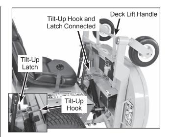
**Deck Secured in TILT-UP Position**
