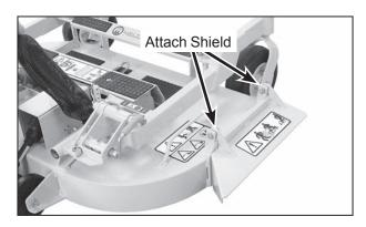
**Deck Discharge Shield Installation**
