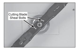
**Cutting Blade Shear Bolts**
