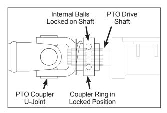
**Quick Disconnect Ring "Locked" Position**
