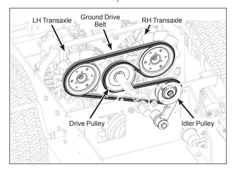
**Ground Drive Belt Assembly (Engaged)**
