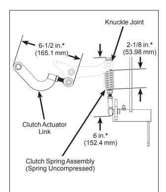
\*NOTE: Factory preset dimensions. Reset to these dimensions prior to adjustment if components have been disassembled.
