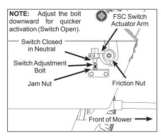
FSC Neutral Switch Adjustment (Side View Through Chassis)
