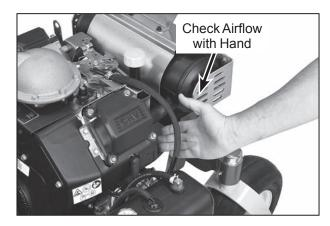
**Cooling System Airflow**
