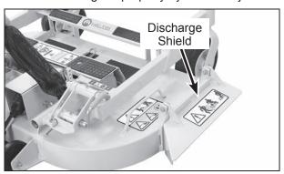
Side Discharge Deflector Shield in **Lowest Position**
