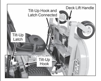
**Deck Secured in TILT-UP Position**
