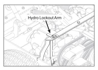
**Hydro Lockout Arm - Normal Operating Position**
