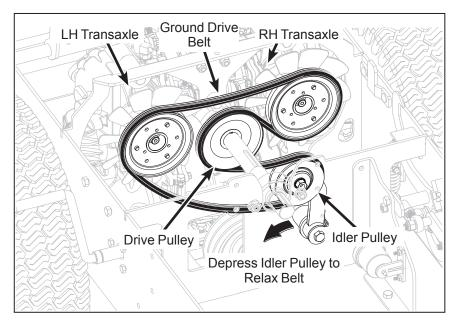
**Ground Drive Belt Assembly (Disengaged)**
