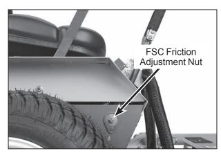
**FSC Friction Adjustment Nut**
