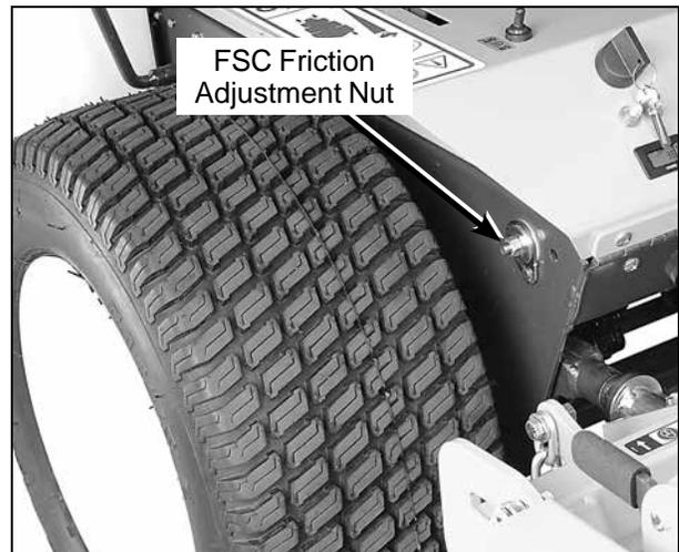
**FSC Adjustment Friction Nut**
