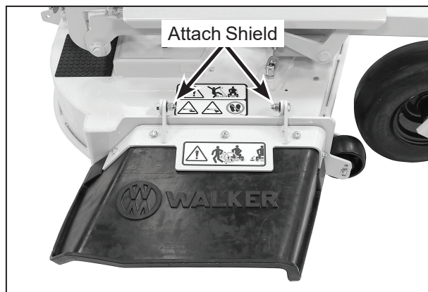
Deck Discharge Shield Installation
