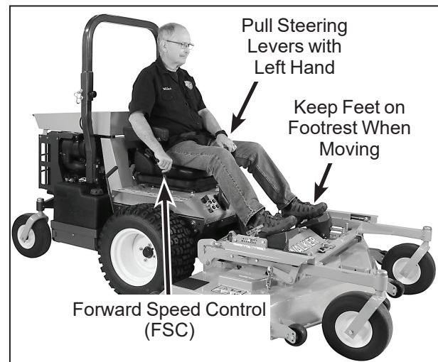
Correct Operator Hand Position on the Controls
