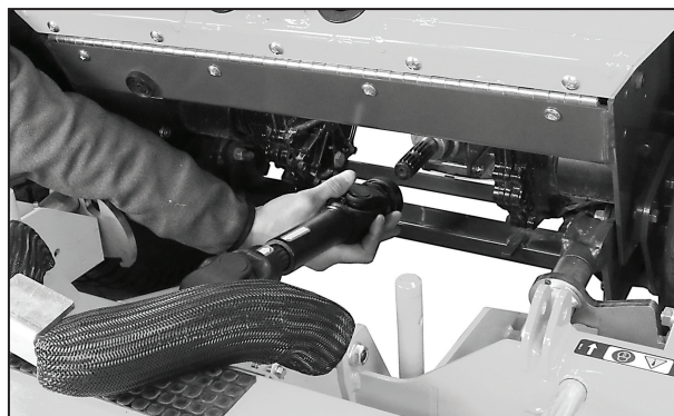
Install PTO Coupler on Tractor PTO Shaft (Shown with Debris Guard Removed for Clarity)
