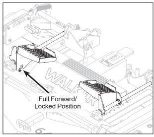
Adjustable Footrest in Full Forward/Locked Position for Deck Tilt-Up
