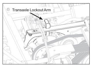
Transaxle Lockout Arm - Freewheel Position
