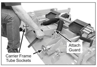
**PTO Shaft Guard Installation**
