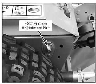
**FSC Friction Adjustment Nut**
