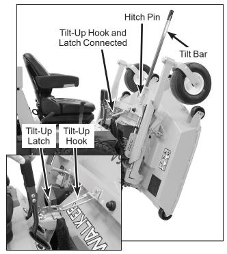
**Deck Secured in TILT-UP Position**
