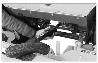
Install PTO Coupler on Tractor PTO Shaft (Shown with Debris Guard Removed for Clarity)
