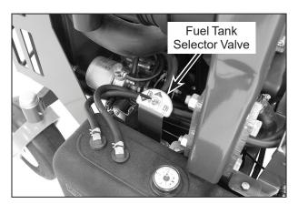
Fuel Tank Selector Valve (RH Side View)
