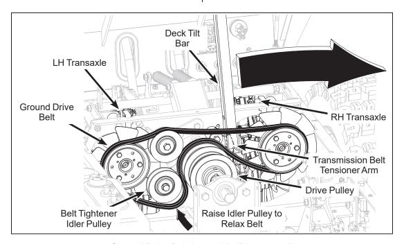
**Ground Drive Belt Assembly (Disengaged)**
