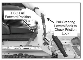
FSC Friction Adjustment Test (Checking Friction Lock)
