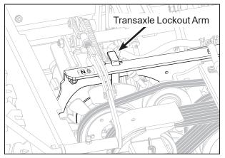
Transaxle Lockout Arm - Normal Operating Position
