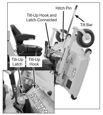
**Deck Secured in TILT-UP Position**
