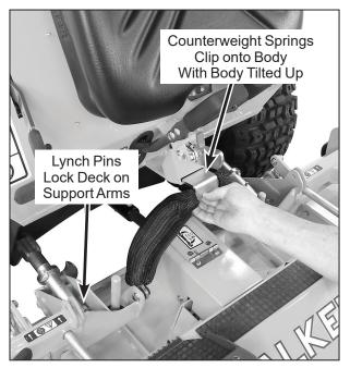
**Deck Counterweight Spring Installation**
