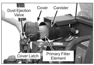
Air Cleaner Components (Shown with Cover Being Removed)
