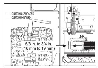
**Clutch Idler Pulley Travel Adjustment**
