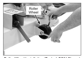
Roller Wheel Installation (Typical, DS61 Shown)
