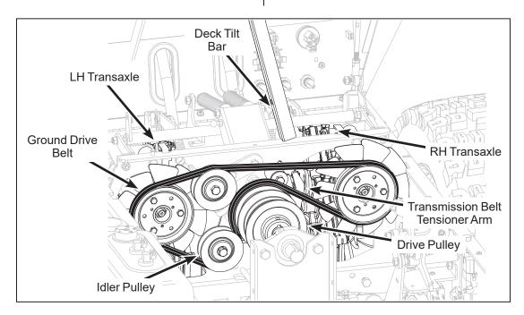
**Ground Drive Belt Assembly (Engaged)**
