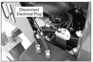
Disconnect Electrical Plug on **Fuel Shut-Off Solenoid**
