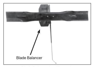
**Blade Balanced on Magnetic** Wall-Mounted Balancer
