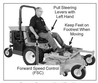
**Correct Operator Hand Position** on the Controls
