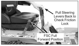
FSC Friction Adjustment Test (Checking Friction Lock)
