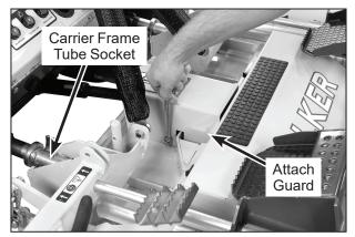
**PTO Shaft Guard Installation**
