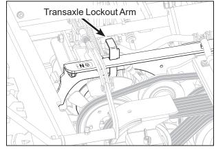
**Transaxle Lockout Arm - Freewheel Position**
