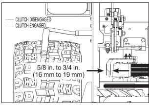
**Clutch Idler Pulley Travel Adjustment**
