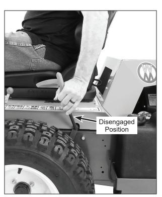
Parking Brake Disengaged
