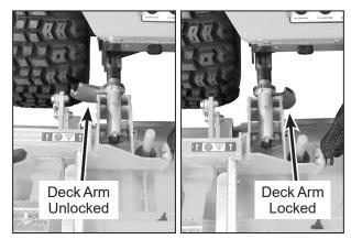
Deck Arms in Unlocked and Locked Positions
