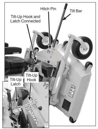
Deck Secured in TILT-UP Position
