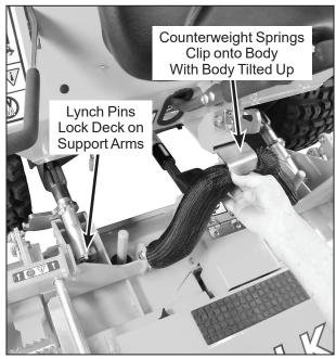
Deck Counterweight Spring Installation
