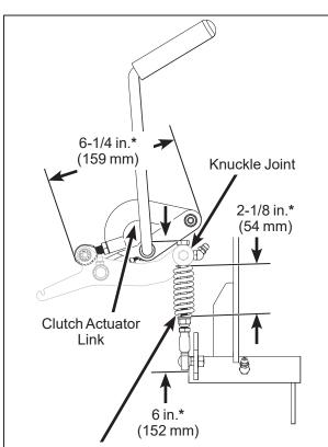
Clutch Spring Assembly (Spring Uncompressed)
