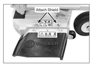
**Deck Discharge Shield Installation**
