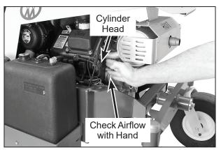
**Check Cooling System Airflow**
