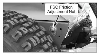
**FSC Friction Adjustment Nut**
