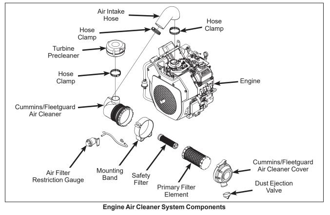
**IMPORTANT:** Use **only** Cummins/Fleetguard air filter elements for replacement (Walker 2090-1 and 2090-3). Aftermarket filters may not seal properly or filter efficiently.
