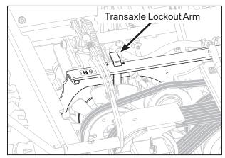
Transaxle Lockout Arm - Normal Operating Position
