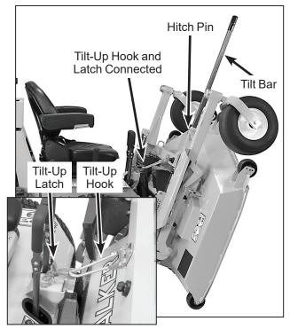
**Deck Secured in TILT-UP Position**
