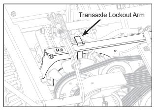
Transaxle Lockout Arm - Normal Operating Position
