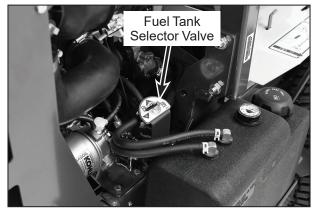
Fuel Tank Selector Valve (RH Side View)
