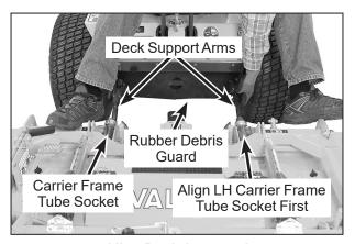
Align Deck Arms and Carrier Frame Tube Sockets
