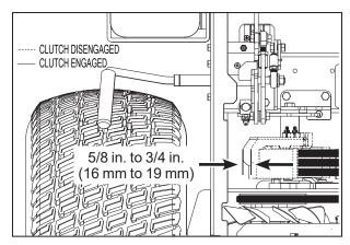
**Clutch Idler Pulley Travel Adjustment**
