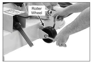
Roller Wheel Installation (Typical, DS61 Shown)
