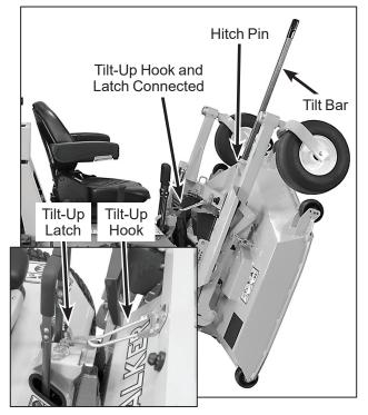
**Deck Secured in TILT-UP Position**
