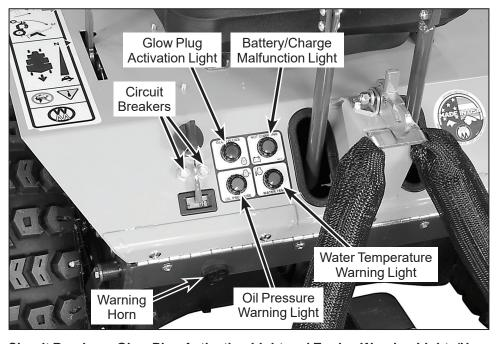
Circuit Breakers, Glow Plug Activation Light and Engine Warning Lights/Horn
