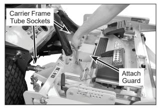
**PTO Shaft Guard Installation**
