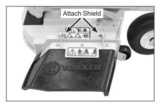
**Deck Discharge Shield Installation**
