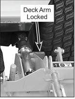
Deck Arms in Unlocked and Locked Positions
