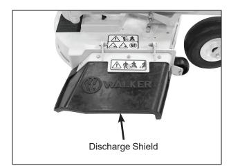
**Side Discharge Deflector Shield in Lowest Position**
