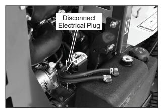
**Disconnect Electrical Plug on Fuel Shut-Off Solenoid**
