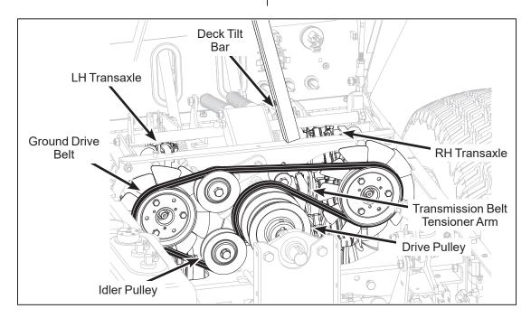
**Ground Drive Belt Assembly (Engaged)**
