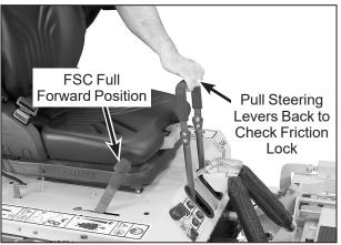
FSC Friction Adjustment Test (Checking Friction Lock)
