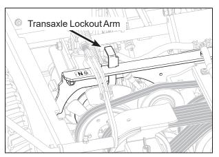
Transaxle Lockout Arm - Freewheel Position
