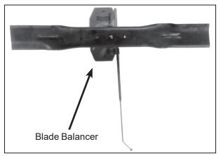
**Blade Balanced on Magnetic** Wall-Mounted Balancer
