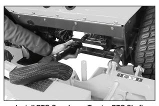
**Install PTO Coupler on Tractor PTO Shaft**
