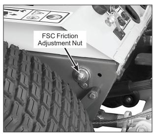
**FSC Friction Adjustment Nut**
