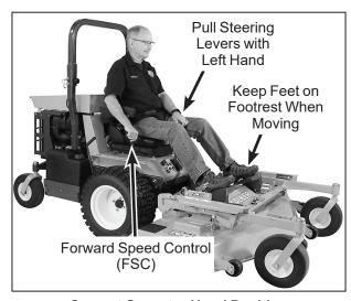
**Correct Operator Hand Position** on the Controls
