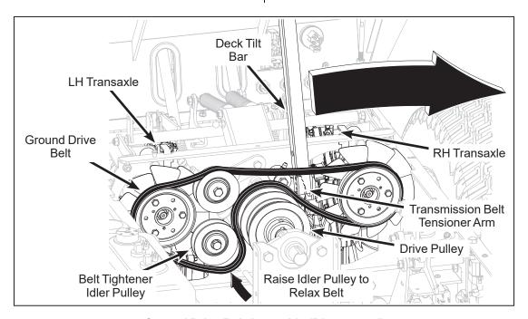
**Ground Drive Belt Assembly (Disengaged)**
