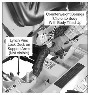
**Deck Counterweight Spring Installation**
