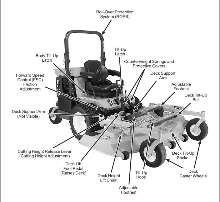
Note: The H24d shown is equipped with the optional All-Terrain Tires.
