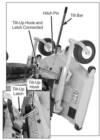
**Deck Secured in TILT-UP Position**
