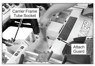
**PTO Shaft Guard Installation**
