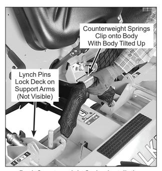
**Deck Counterweight Spring Installation**
