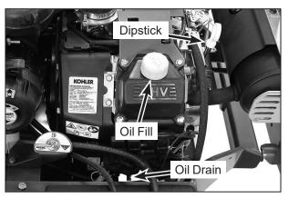
Dipstick, Oil Fill and Oil Drain Locations (View from Above Left Side of Tractor)
