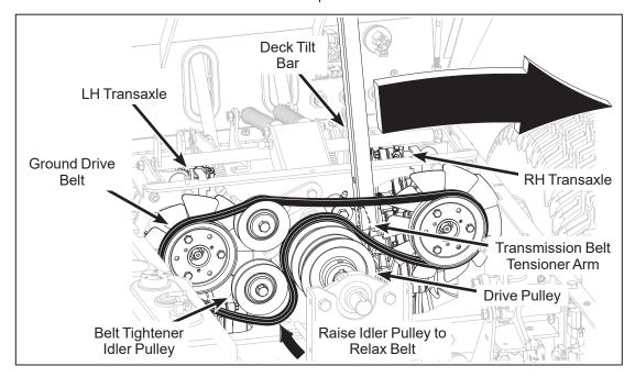
**Ground Drive Belt Assembly (Disengaged)**
