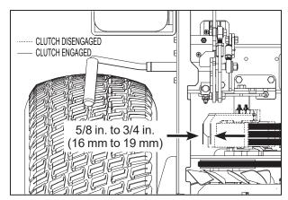
**Clutch Idler Pulley Travel Adjustment**
