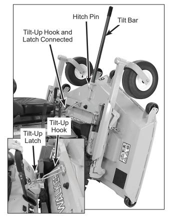
**Deck Secured in TILT-UP Position**
