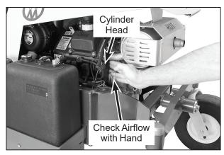
**Check Cooling System Airflow**
