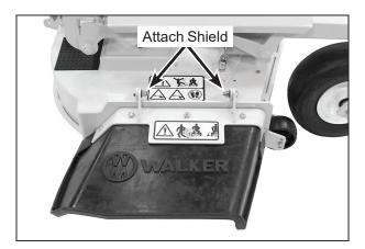
**Deck Discharge Shield Installation**
