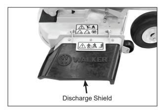
**Side Discharge Deflector Shield in Lowest Position**
