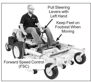
**Correct Operator Hand Position** on the Controls
