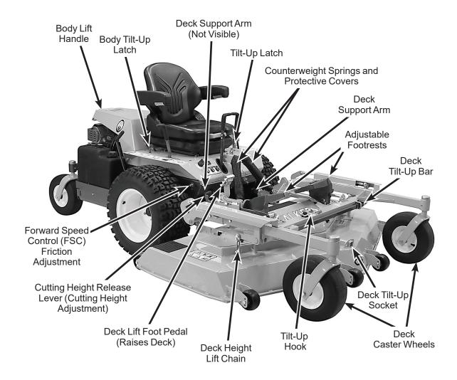
**NOTE:** The H27i shown is equipped with the optional All-Terrain Tires.
