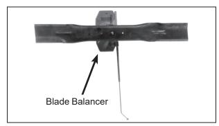
Blade Balanced on Magnetic Wall-Mounted Balancer
