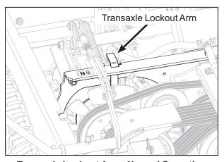
Transaxle Lockout Arm - Normal Operating Position
