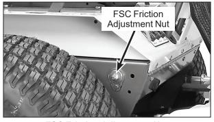
**FSC Friction Adjustment Nut**
