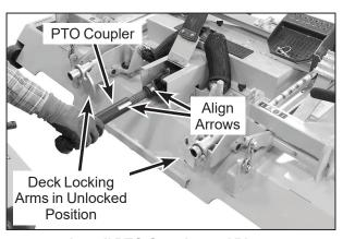
Install PTO Coupler and Place Deck Locking Arms in Unlocked Position
