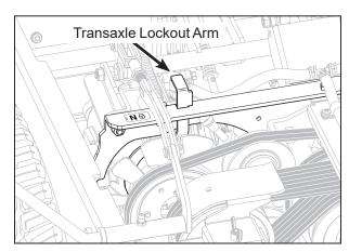
**Transaxle Lockout Arm - Freewheel Position**
