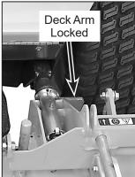
**Deck Arms in Unlocked and Locked Positions**
