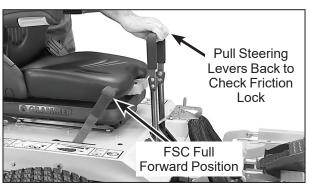
**FSC Friction Adjustment Test** (Checking Friction Lock)
