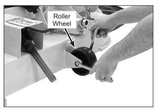
Roller Wheel Installation (Typical, DS61 Shown)
