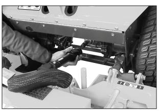
**Install PTO Coupler on Tractor PTO Shaft**
