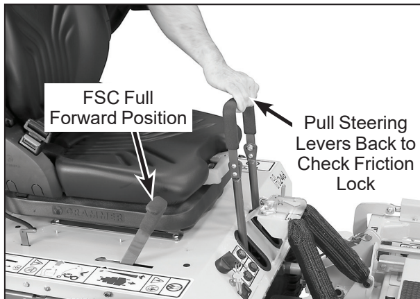
FSC Friction Adjustment Test (Checking Friction Lock)
