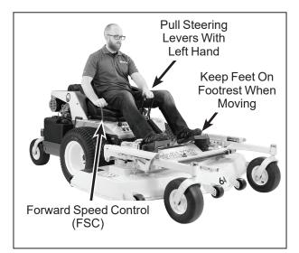
**Correct Operator Hand Position** on the Controls
