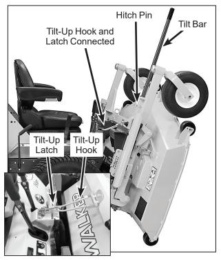
**Deck Secured in TILT-UP Position**
