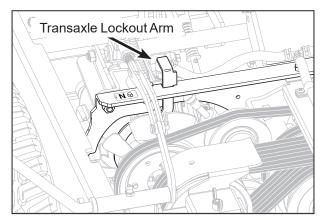
Transaxle Lockout Arm - Freewheel Position
