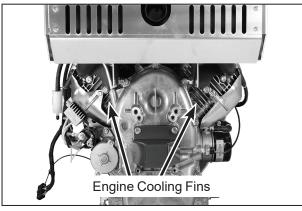
**Inspect Cylinder Head Cooling Fins** (Viewed from Rear of Engine)
