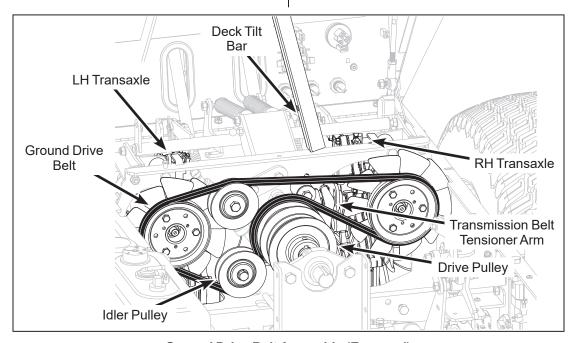
**Ground Drive Belt Assembly (Engaged)**
