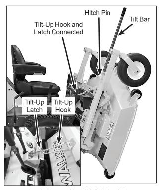
**Deck Secured in TILT-UP Position**
