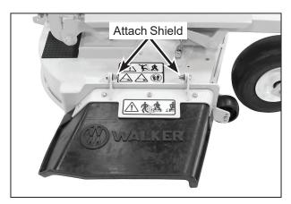
**Deck Discharge Shield Installation**
