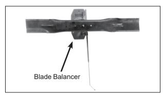
**Blade Balanced on Magnetic Wall-Mounted Balancer**
