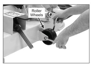
Roller Wheel Installation (Typical, DS61 Shown)
