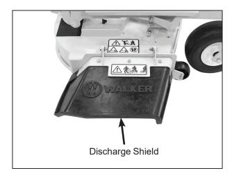
Side Discharge Deflector Shield in Lowest Position
