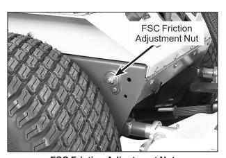
**FSC Friction Adjustment Nut**
