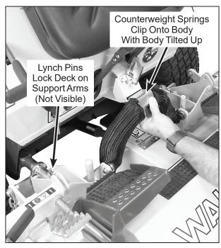
**Deck Counterweight Spring Installation**
