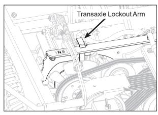
Transaxle Lockout Arm - Normal Operating Position
