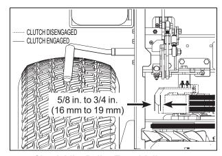
**Clutch Idler Pulley Travel Adjustment**
