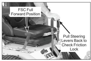
FSC Friction Adjustment Test (Checking Friction Lock)
