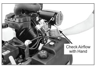
**Check Cooling System Airflow**
