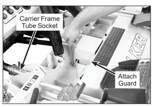
**PTO Shaft Guard Installation**
