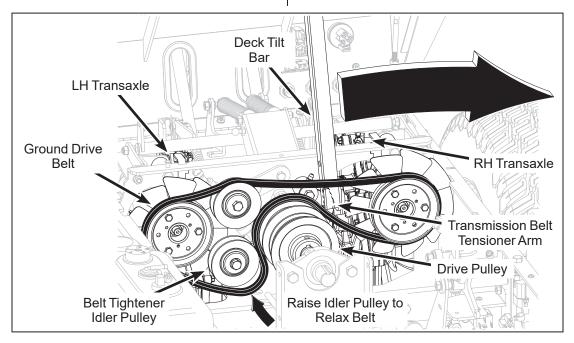
**Ground Drive Belt Assembly (Disengaged)**
