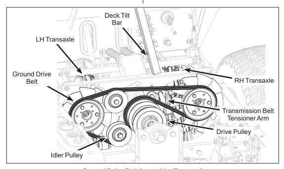
**Ground Drive Belt Assembly (Engaged)**
