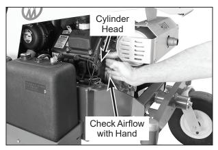
**Check Cooling System Airflow**
