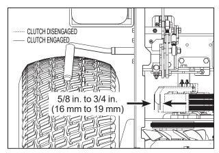
**Clutch Idler Pulley Travel Adjustment**
