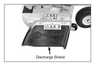
**Side Discharge Deflector Shield in Lowest Position**
