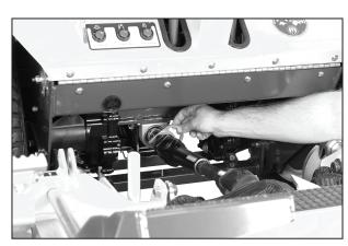
Coupler Installation Tool Removal (Shown with Debris Guard Removed for Clarity)
