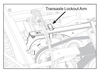
Transaxle Lockout Arm - Normal Operating Position
