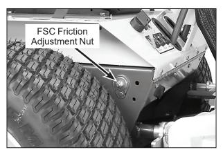
**FSC Friction Adjustment Nut**
