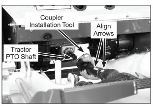
PTO Shaft Connection (Shown with Debris Guard Removed for Clarity)
