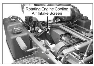
Keep Rotating Engine Cooling Air Intake Screen Clean
