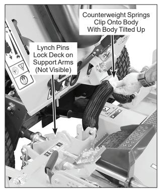
**Deck Counterweight Spring Installation**
