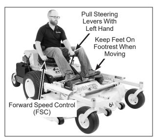
**Correct Operator Hand Position** on the Controls
