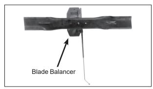
Blade Balanced on Magnetic Wall-Mounted Balancer
