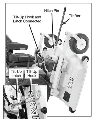
Deck Secured in TILT-UP Position
