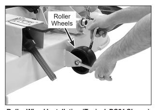
Roller Wheel Installation (Typical, DS61 Shown)
