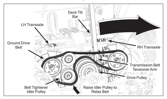
**Ground Drive Belt Assembly (Disengaged)**
