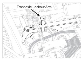
Transaxle Lockout Arm - Freewheel Position
