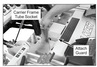
**PTO Shaft Guard Installation**
