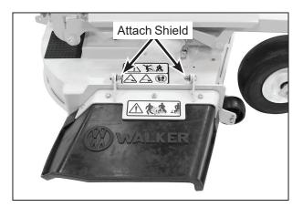
**Deck Discharge Shield Installation**
