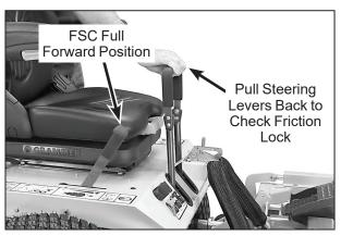
FSC Friction Adjustment Test (Checking Friction Lock)
