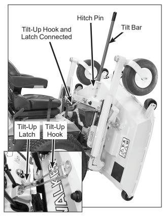
**Deck Secured in TILT-UP Position**
