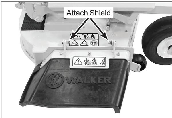
**Deck Discharge Shield Installation**
