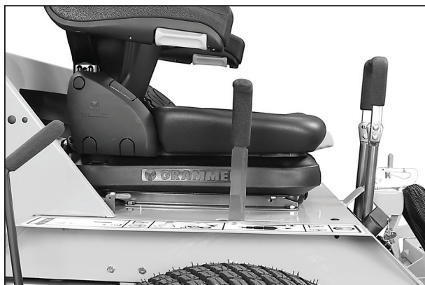
Correct FSC Lever NEUTRAL-PARK Position
