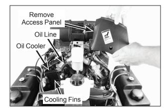
Engine Cylinder Head Access Panels Removed
