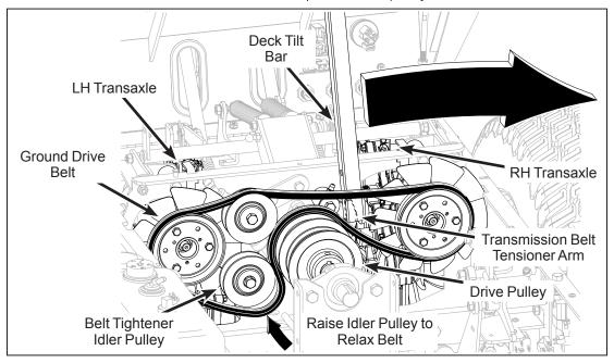
**Ground Drive Belt Assembly (Disengaged)**
