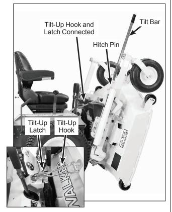
**Deck Secured in TILT-UP Position**
