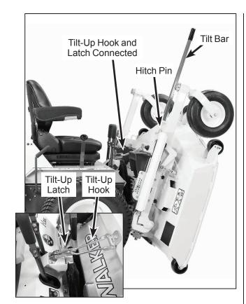
**Deck Secured in TILT-UP Position**
