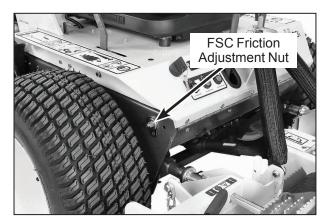
**FSC Friction Adjustment Nut**
