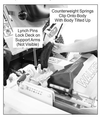
**Deck Counterweight Spring Installation**
