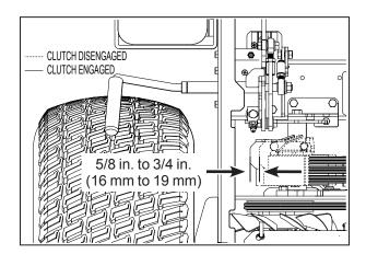
**Clutch Idler Pulley Travel Adjustment**
