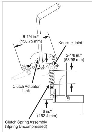
**\*NOTE:** Factory preset dimensions. Reset to these dimensions prior to adjustment if components have been disassembled.
