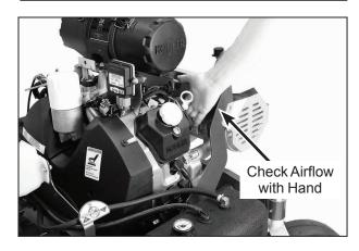
**Check Cooling System Airflow**
