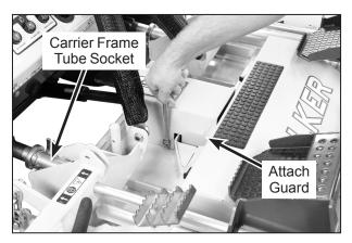
**PTO Shaft Guard Installation**
