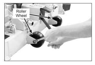
Roller Wheel Installation (Typical, DS60 Shown)
