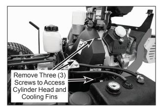
Remove Cylinder Head Access Panel(s) to Clean Cooling Fins
