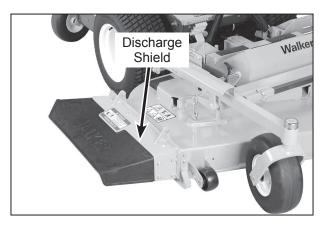
Side Discharge Deflector Shield in Lowest Position
