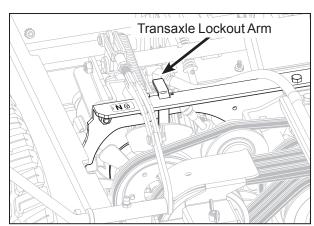
Transaxle Lockout Arm - Normal Operating Position
