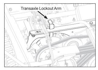
Transaxle Lockout Arm - Freewheel Position
