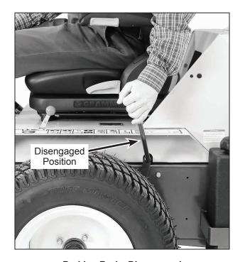
Parking Brake Disengaged
