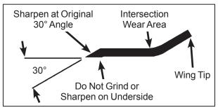
**Mower Blade Profile for Sharpening**
