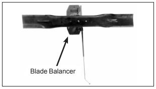
Blade Balanced on Magnetic Wall-Mounted Balancer
