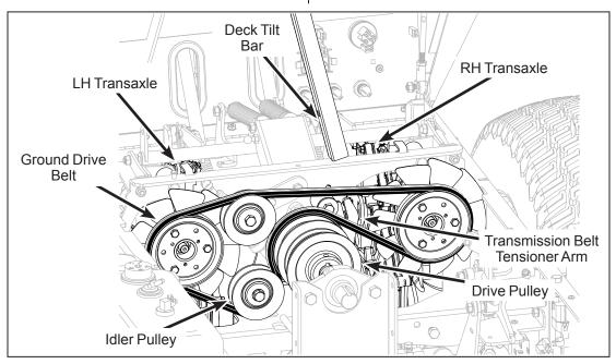
**Ground Drive Belt Assembly (Engaged)**
