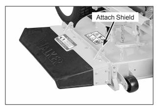
**Deck Discharge Shield Installation**
