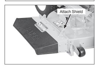
**Deck Discharge Shield Installation**
