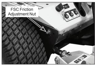
**FSC Friction Adjustment Nut**
