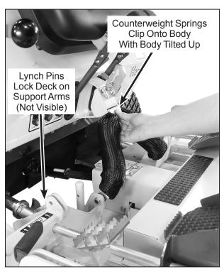
**Deck Counterweight Spring Installation**
