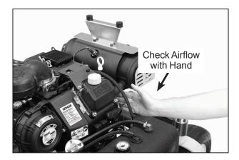
**Check Cooling System Airflow**
