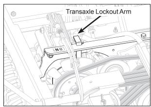
Transaxle Lockout Arm - Normal Operating **Position**
