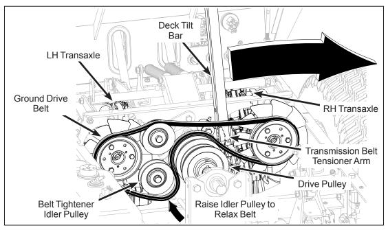
**Ground Drive Belt Assembly (Disengaged)**
