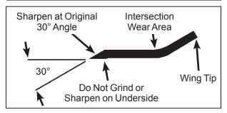
**Mower Blade Profile for Sharpening**
