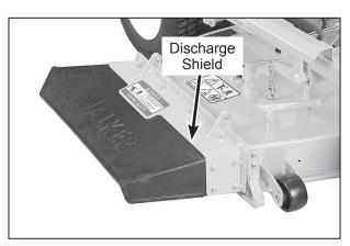
Side Discharge Deflector Shield in Lowest Position
