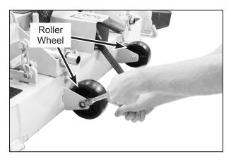
Roller Wheel Installation (Typical, DS60 Shown)
