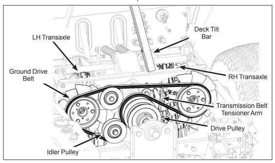
**Ground Drive Belt Assembly (Engaged)**
