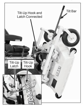
**Deck Secured in TILT-UP Position**
