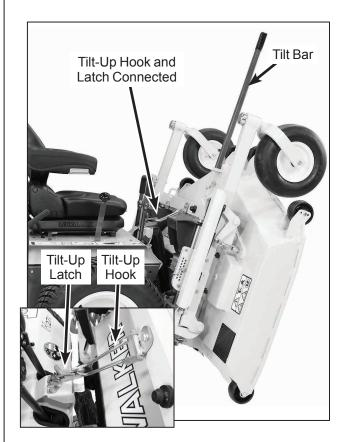
**Deck Secured in TILT-UP Position**
