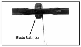
**Blade Balanced on Magnetic Wall-Mounted Balancer**
