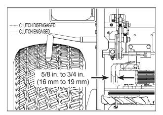
**Clutch Idler Pulley Travel Adjustment**
