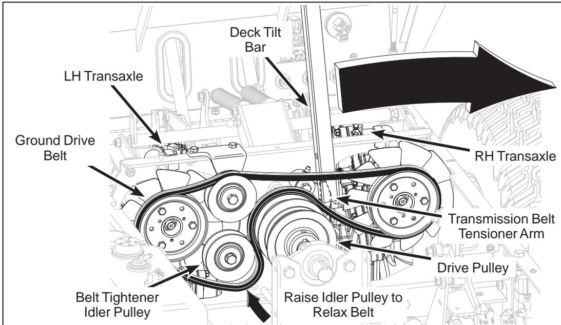
**Ground Drive Belt Assembly (Disengaged)**
