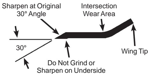
**Mower Blade Profile for Sharpening**
