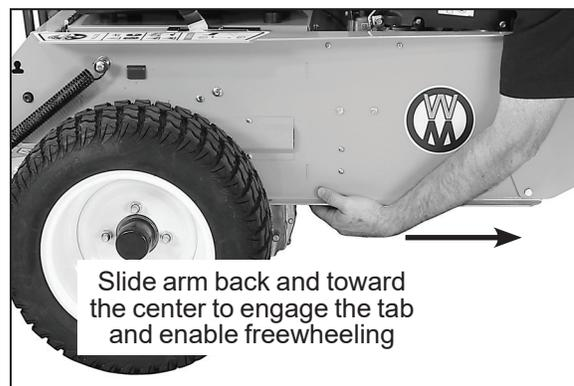
Engage Transaxle LOCKOUT (LH shown)
