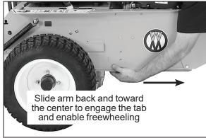
Engage Transaxle LOCKOUT (LH shown)
