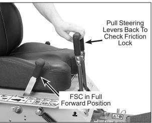
**FSC Friction Adjustment Test**
