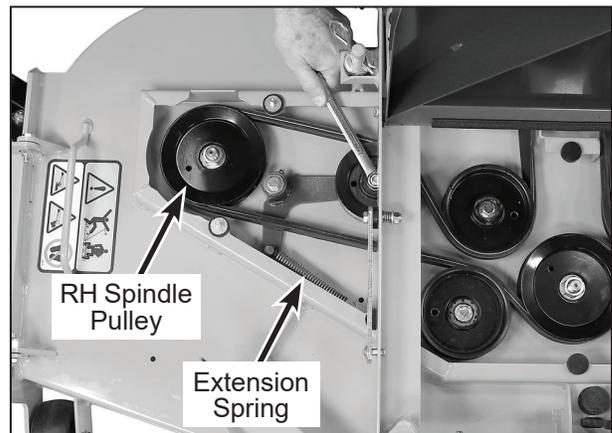
**54" Deck: Remove Belt from RH Spindle Pulley**
