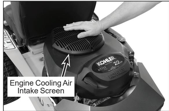
**Checking Engine Air Flow**
