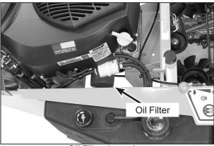
Oil Filter Location (Beneath the Fuel Filter)
