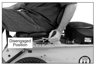
Parking Brake Disengaged
