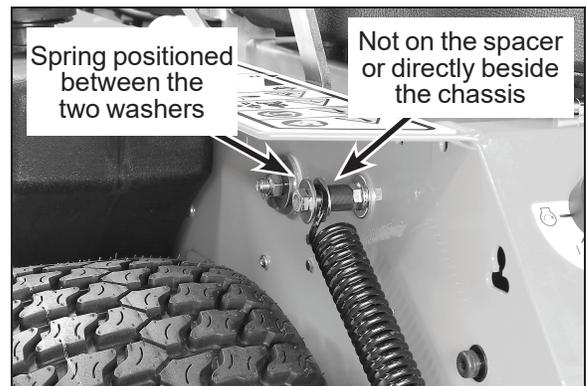
Counterweight Spring Installed on Tractor Post
