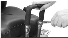
Steering Lever Handles Installed
