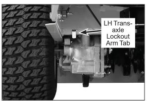
LH Transaxle Lockout Arm Tab
