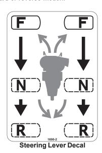
The Forward Speed Control (FSC) lever sets the maximum forward speed, and also sets the forward position of the steering levers.
