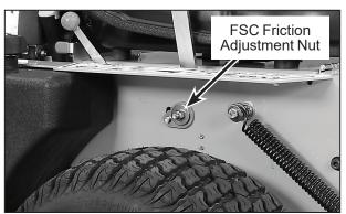
**FSC Friction Adjustment Nut**
