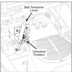
Unlock and Disengage Belt Tensioner Lever
