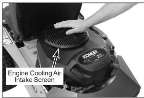
**Checking Engine Air Flow**
