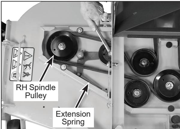
**54" Deck: Removing Belt from RH Spindle Pulley**
