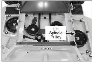
42", 48" Deck: Remove Belt from LH Spindle Pulley
