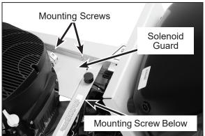
**Remove Solenoid Guard for Clutch Wire Access**
