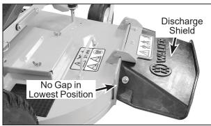
Side Discharge Shield in Lowest Position
