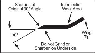
**Mower Blade Profile for Sharpening**
