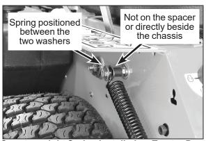
**Counterweight Spring Installed on Tractor Post**
