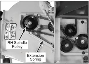
54" Deck: Removing Belt from RH Spindle Pulley
