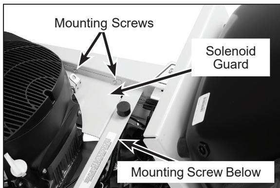
**Remove Solenoid Guard for Clutch Wire Access**
