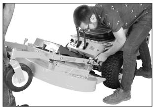
Install Counterweight Spring on Carrier Frame
