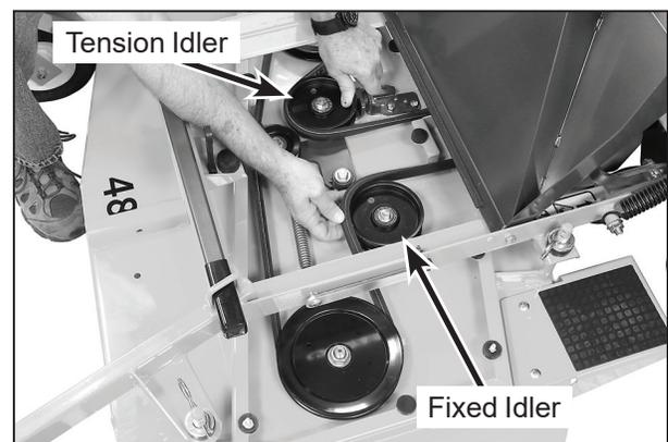
42", 48" Deck: Removing Belt from LH Idler Pulley
