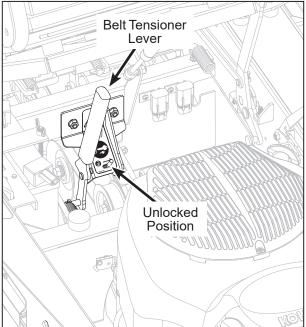
Unlock and Disengage Belt Tensioner Lever
