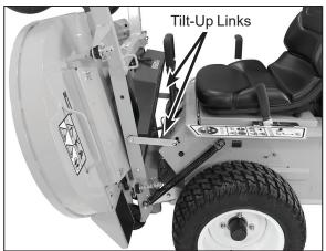
**Deck Locked in Tilt-Up Position**
