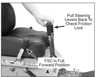
**FSC Friction Adjustment Test**
