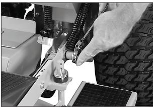
**Install Nut on Carriage Bolt**
