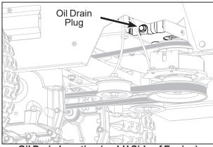
Oil Drain Location (on LH Side of Engine)
