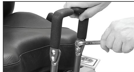
**Steering Lever Handles Installed**
