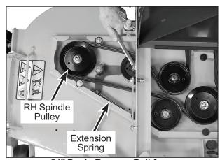
54" Deck: Remove Belt from RH Spindle Pulley
