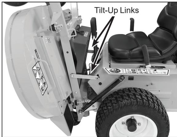
Deck Locked in Tilt-Up Position
