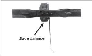
Blade Balanced on Magnetic Wall-Mounted **Balancer**
