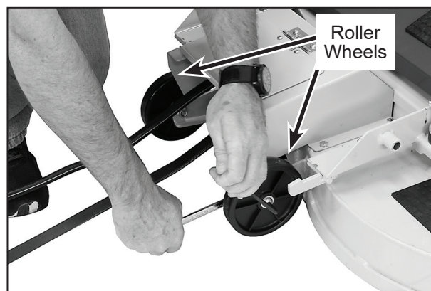
Roller Wheel Installation
