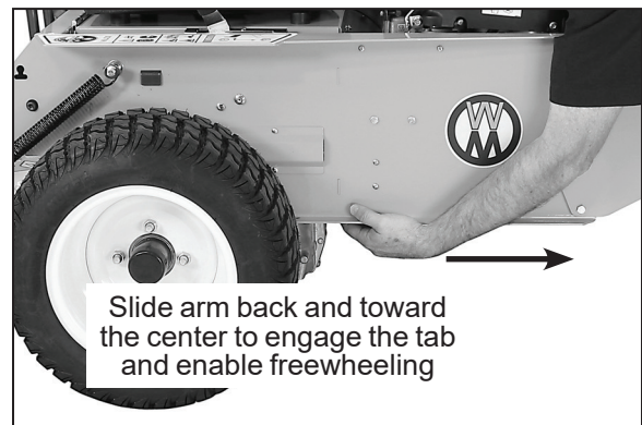
Engage Transaxle LOCKOUT (LH shown)
