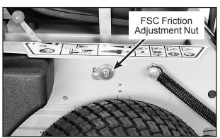
**FSC Friction Adjustment Nut**
