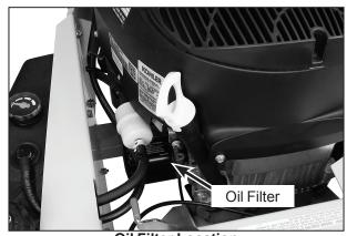
Oil Filter Location (Beneath the Fuel Filter)
