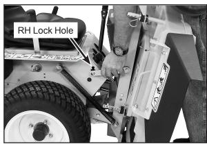
Insert RH and LH Tilt-Up Links into the **Lock Holes**
