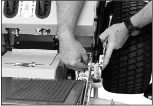
**Install Nut on Carriage Bolt**
