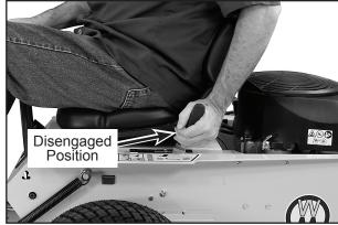
Parking Brake Disengaged
