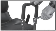
**Steering Lever Handles Installed**
