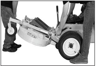
**Install Counterweight Spring on Carrier Frame**
