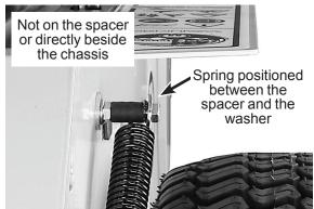
**Counterweight Spring Installed on Tractor Post**
