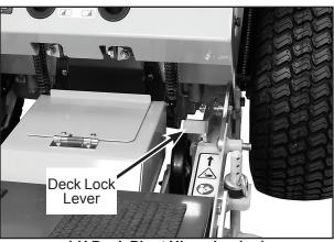
**LH Deck Pivot Hinge Locked**
