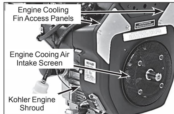
**Engine Cooling Air Intake Screen and Cooling Fin Access Panels**
