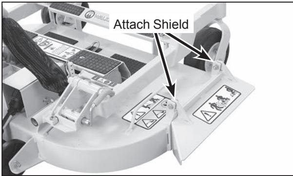
**Deck Discharge Shield Installation**
