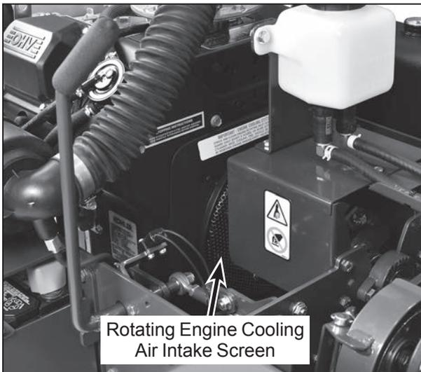
**Keep Rotating Engine Cooling Air Intake Screen Clean**
