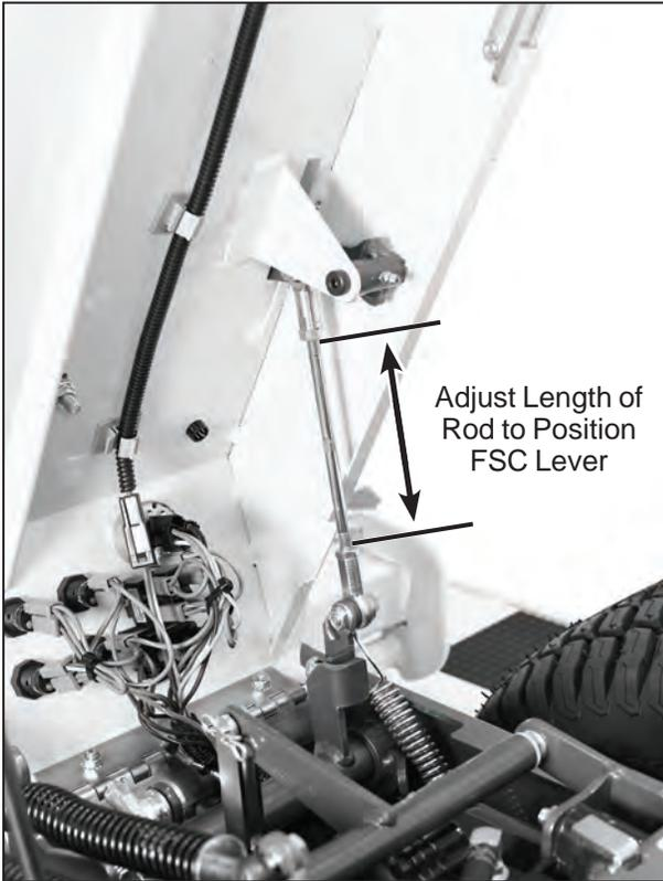
Adjust Length of Rod to Position FSC Lever
